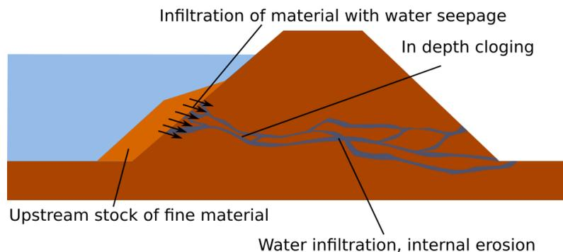
Figure 1: Field technique to inject fine material into a degraded earthen hydraulic structure.
