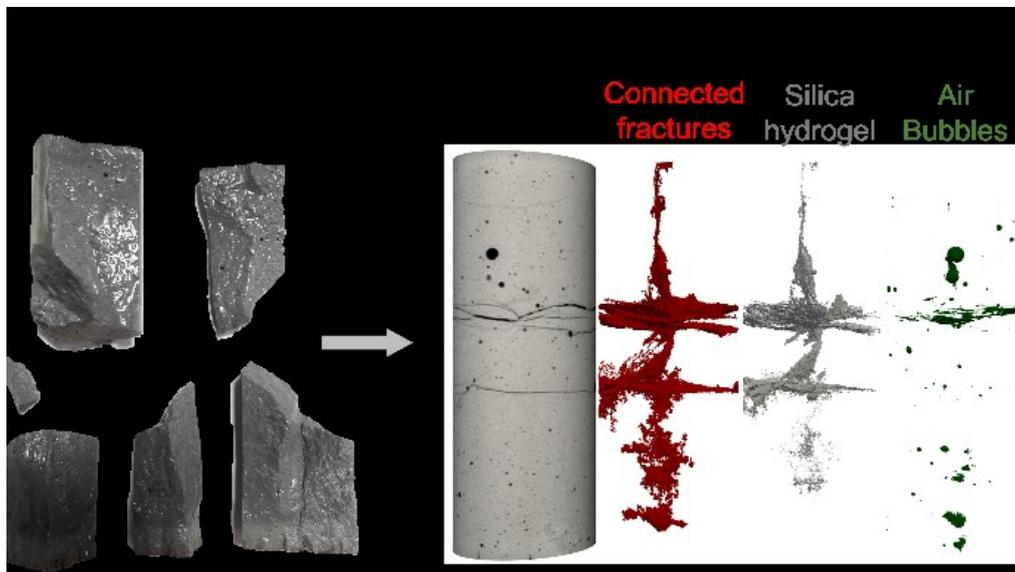
*Figure 1. A fractured rock core repaired using colloidal silica. Figure shows Micro X-CT Images of: the original fracture network; the silica grout in the sample after injection; the remaining air-filled voids.*
