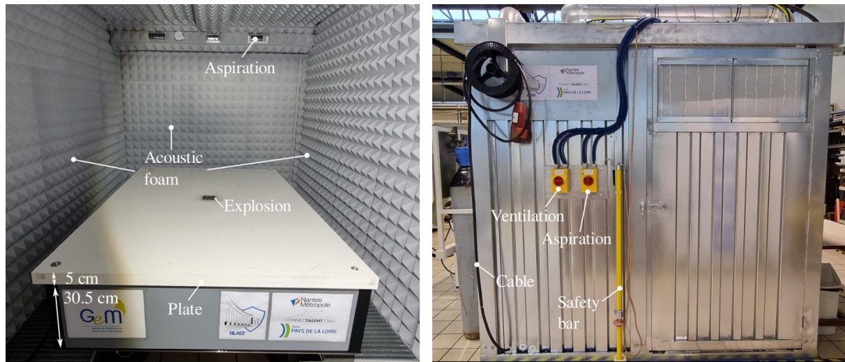
Figure 1: Experimental setup of reduced scale experiments installed in the GeM research laboratory.
