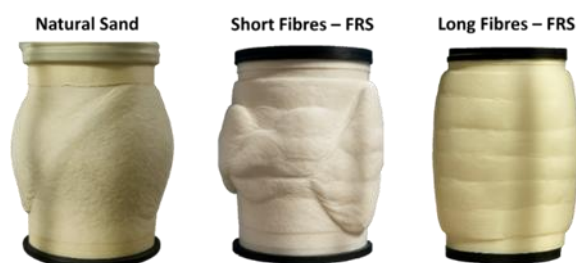
Figure 1: Different soil failure mechanisms: end-of-test configurations of triaxial compression samples under 100 kPa confining pressure — Natural Sand, Fibre-Reinforced Sand with short horizontal fibres (1 cm), and Fibre-Reinforced Sand with long horizontal fibres (6.5 cm).
